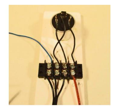
Once I have it wired, I use black 3-strand wire from 022C switch controllers so the exposed wires at the signal look good.
