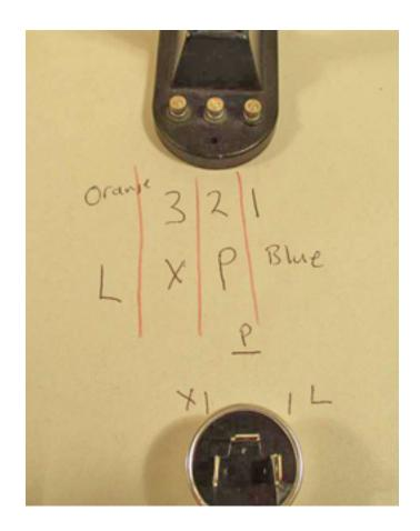
Wiring it the way I have with the blue wire from the insulated rail to the highway flasher ground means if the sign touches the track it will activate rather than cause a short.
