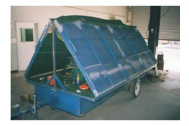
Here is the modified trailer with wings folded. Footnote: The original trailer wheels were the smaller, trailer sized wheels. Unfortunately, that limited towing speed. The solution was to replace the small wheels with regular wheels. The problem was that the spare was mounted on the underside of one wing and thus under its tarp. That was not an option for the larger wheel thus a cradle was made for it and the spare is stored inside the layout bolted to one of the end supports.
