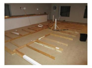
There is a 36" wide aisle. Then there is a 13 foot wide by 26' 8" O gauge layout 5" off the floor with a 4 by 6 foot extension in the southwest corner for a passenger station area.
