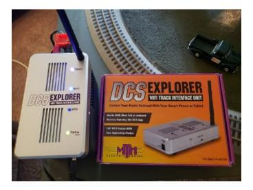
The DCS Explorer sitting on top a MTH Z1000. All that is needed is to put the Explorer between the track and the transformer.
