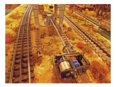
The big obstacle was attaching a 3/8 inch diameter threaded rod to a 1/8 inch diameter motor shaft. Using a plastic disc, reinforced with a small metal plate, a set of very small machine screws and ample amounts of Gorilla glue seems to be handling the torque just fine. The motor's rpm moves the crane at a fairly good pace with very little power.
